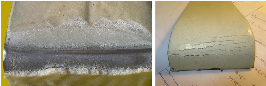
Figure 1: Mirteq's custom made primer. A coated steel plate was bent 90° to fracture the MIR-950 structural coating. The coating was then ground away to expose and show off the tenacious chemical bond the MIR-900 steel primer forms with the steel.
