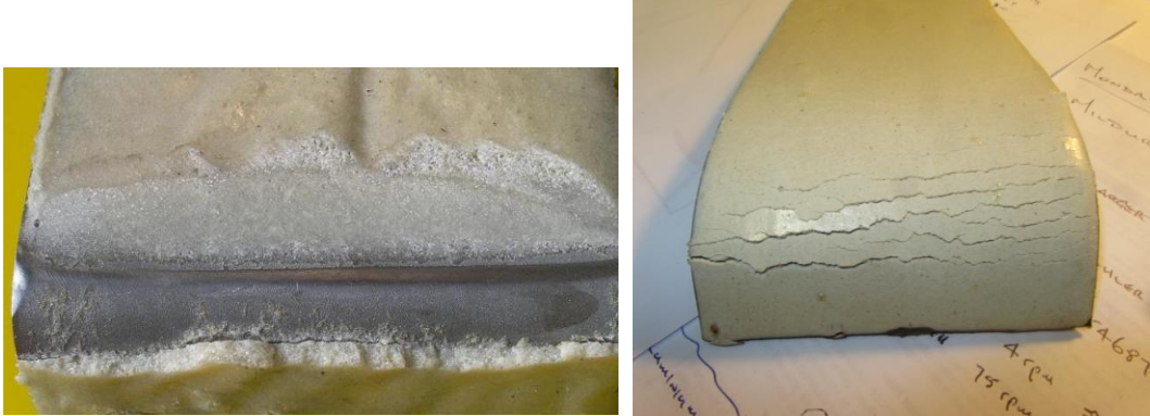
Figure 4: Mirteq's custom made primer. Coated steel plate was bent 90° to fracture the MIR-950 coating. The coating was then ground away to expose and show off the tenacious chemical bond.
